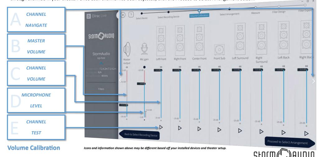
It is now time to acquire the acoustical models by measuring the sound system in the listening room. The accuracy of the models is very important for designing optimal room correction filters. On this screen, the correct seating arrangement needs to be selected.
