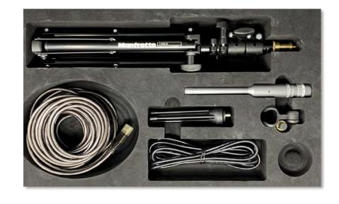
Use a stand that allows you to vary the height of the microphone position within the listening volume, which is important to get an accurate acoustical model. Two types of stand are provided in the integrator kit for maximum flexibility.
